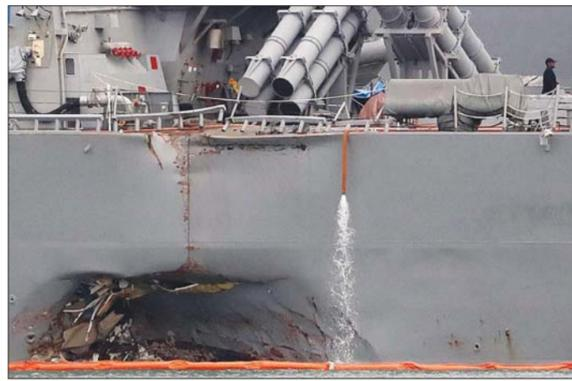
The damaged port aft hull of the USS John S. McCain, is visible while docked at Singapore's Changi naval base Tuesday.
